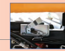
▲ Vessel clearance detect sensor
