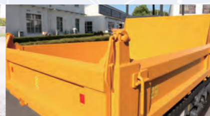
▲Sloped vessel frame
