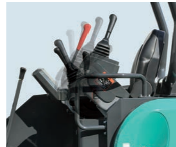
All operations are blocked when the lever is raised.
