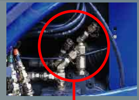
Oil pressure measurement port with quick coupler
