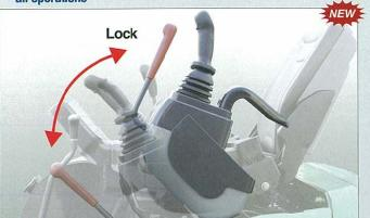
The master gate lock system enables you to block up all functions such as boom, arm, bucket, swing, boom swing, travel and blade.
