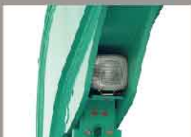
Boom's built-in lamp
