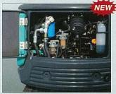
The fully opening engine cover achives simply maintenance. And the radiator and oil cooler are made of aluminum for super corrosion resistance.
