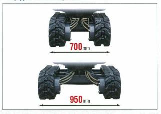
With the widest ranging spanners in its class, the machine can access into tight spaces to ensure a very high level of work performance.
