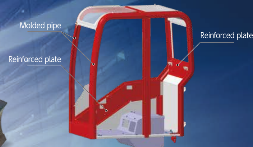
ISO compliant ROPS cab
