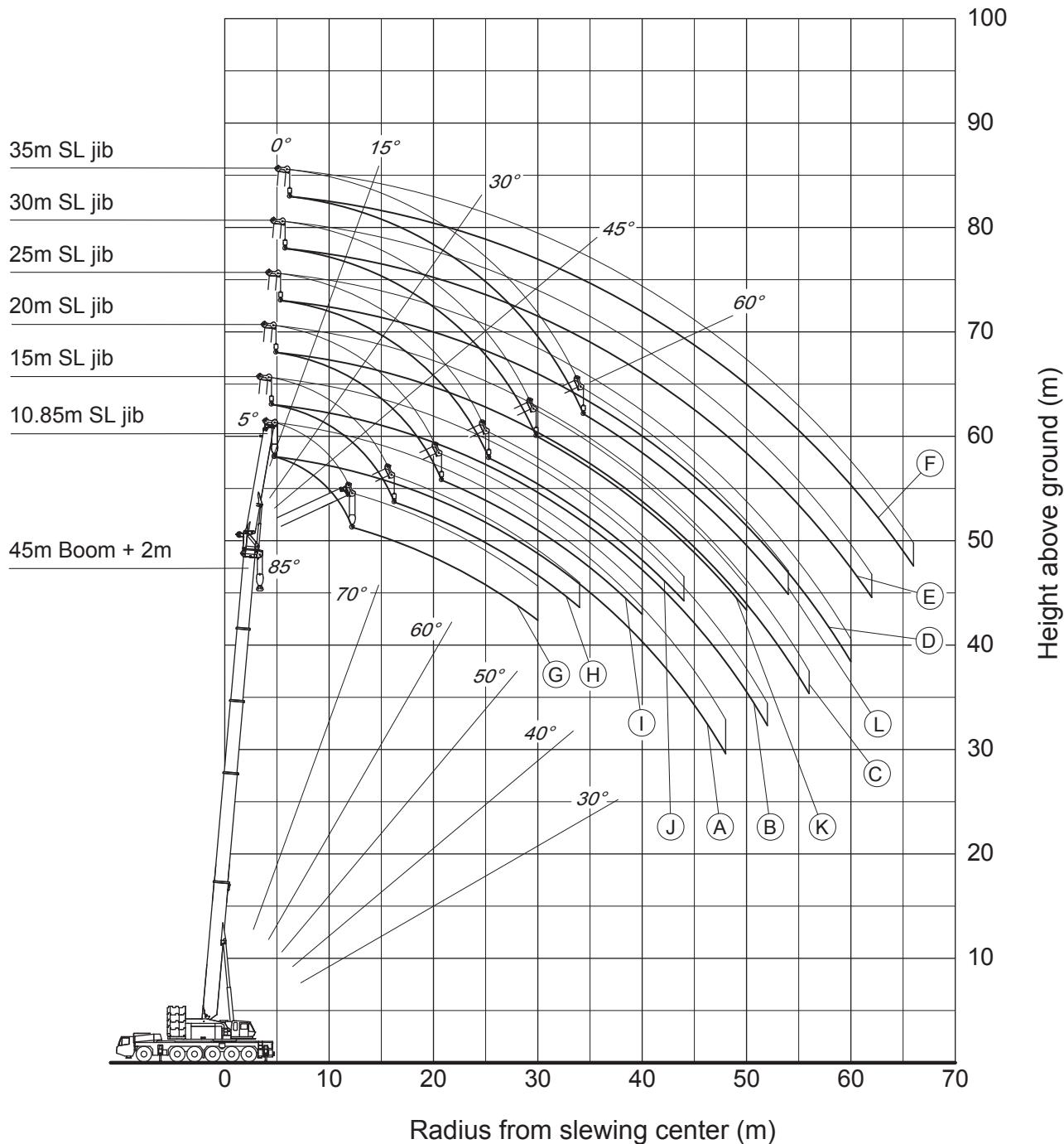
Note: 1. This diagram does not include deflection of Boom and SL jib.
