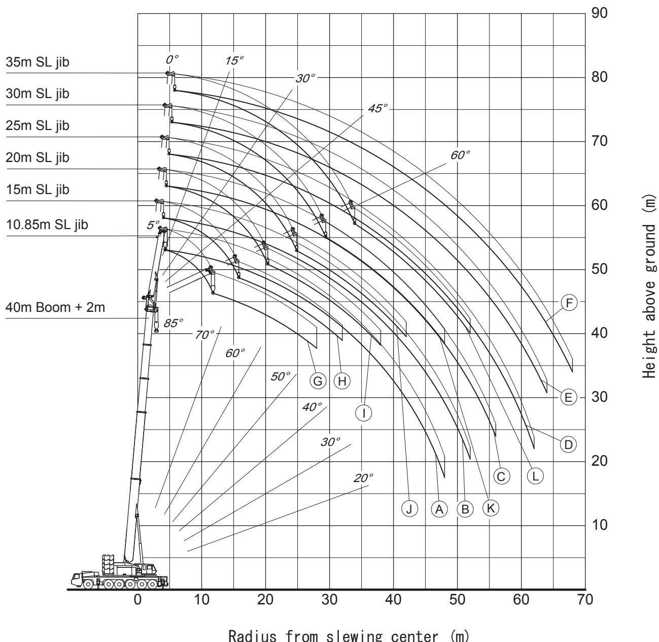
Note: 1. This diagram does not include deflection of Boom and SL jib.
