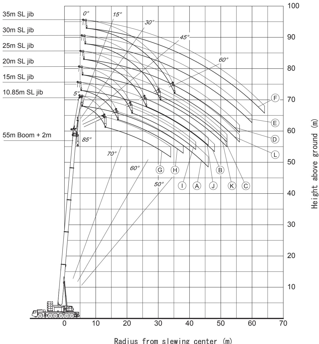
Note: 1. This diagram does not include deflection of Boom and SL jib.
