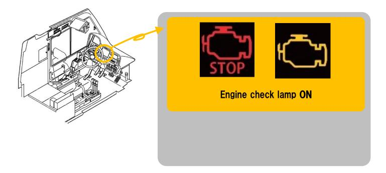
ECU error codes are displayed in the initial screen that appears when the test mode is started in the information display Only error codes for currently active are displayed. A diagnostic tool is required to check the location of past failures or clear the failure history.
