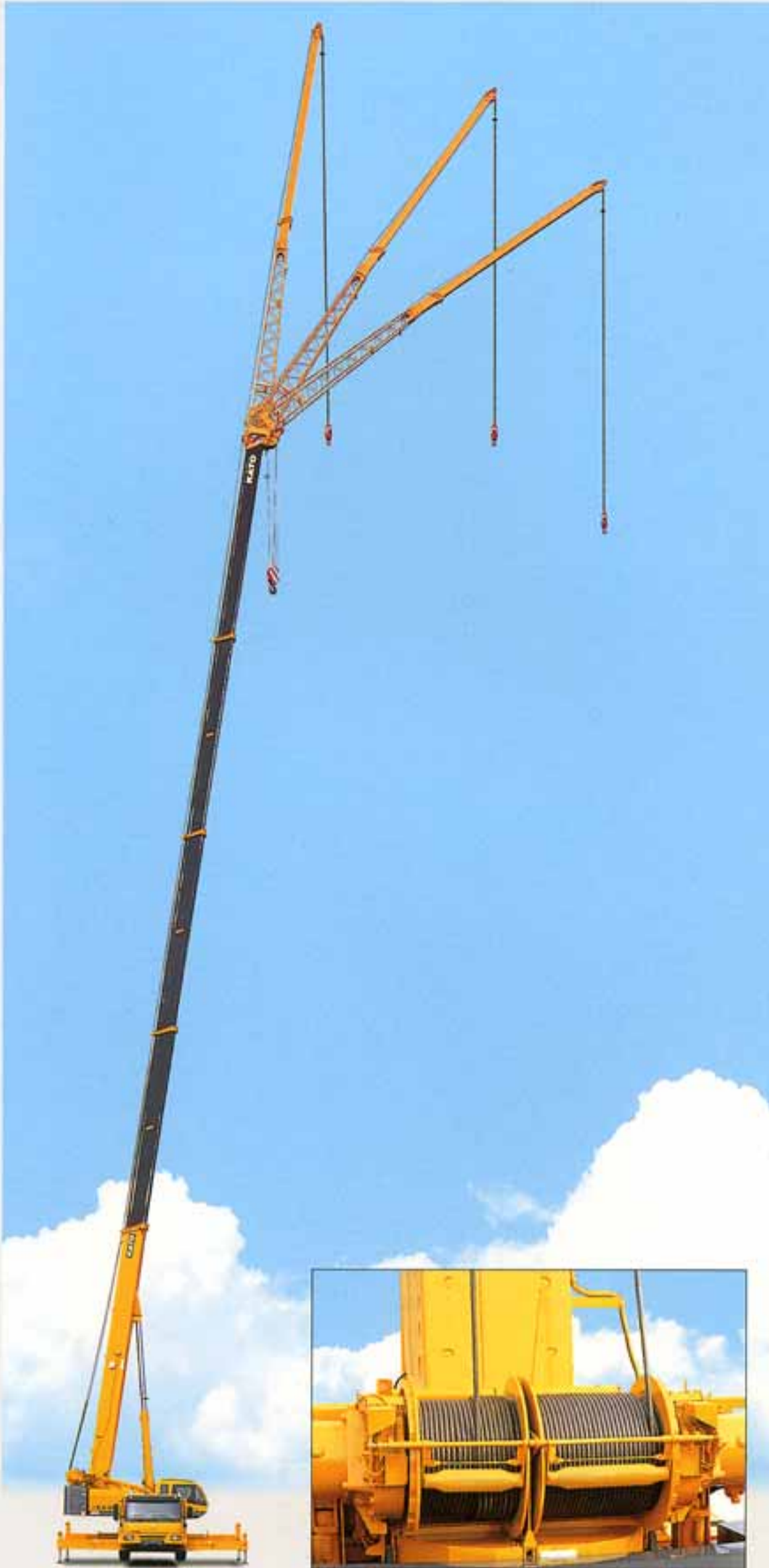
Main & auxiliary winches. Both main & auxiliary winches are built in as standard with a line pull of 6.5tonnes.
