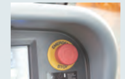
▲ Emergency engine stop switch (for crane operation)
