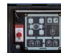
▲ Outriggers control box
