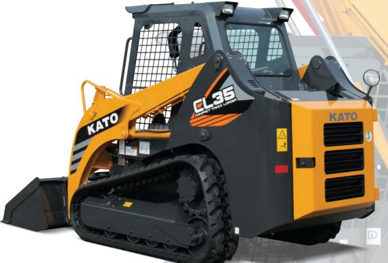
The ROPS can be tilted for easy access to the engine and other service ports.
