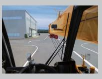
Making front view wider and assuring more safety at travelling with lower position of boom foot pin and smaller front overhang
