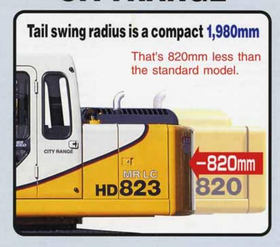
We've pulled the tail swing radius way in, but this machine handles big work. It's just the ticket for tight spaces.
